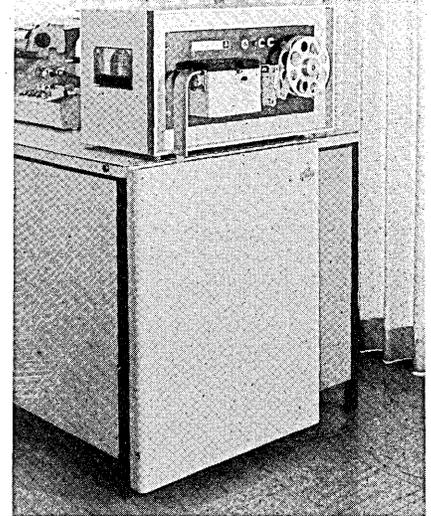
speed of 600 characters per second, or approximately 300 characters per second when stopping on a character with the RECOMP III. The 510 includes such features as printed circuitry, simplified load and unload
