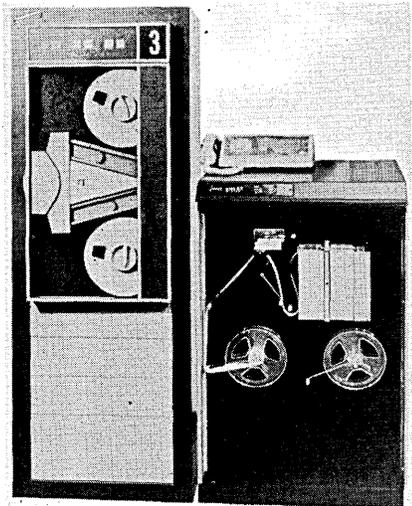
Lateral and longitudinal parity checking with automatic back-up and re-
