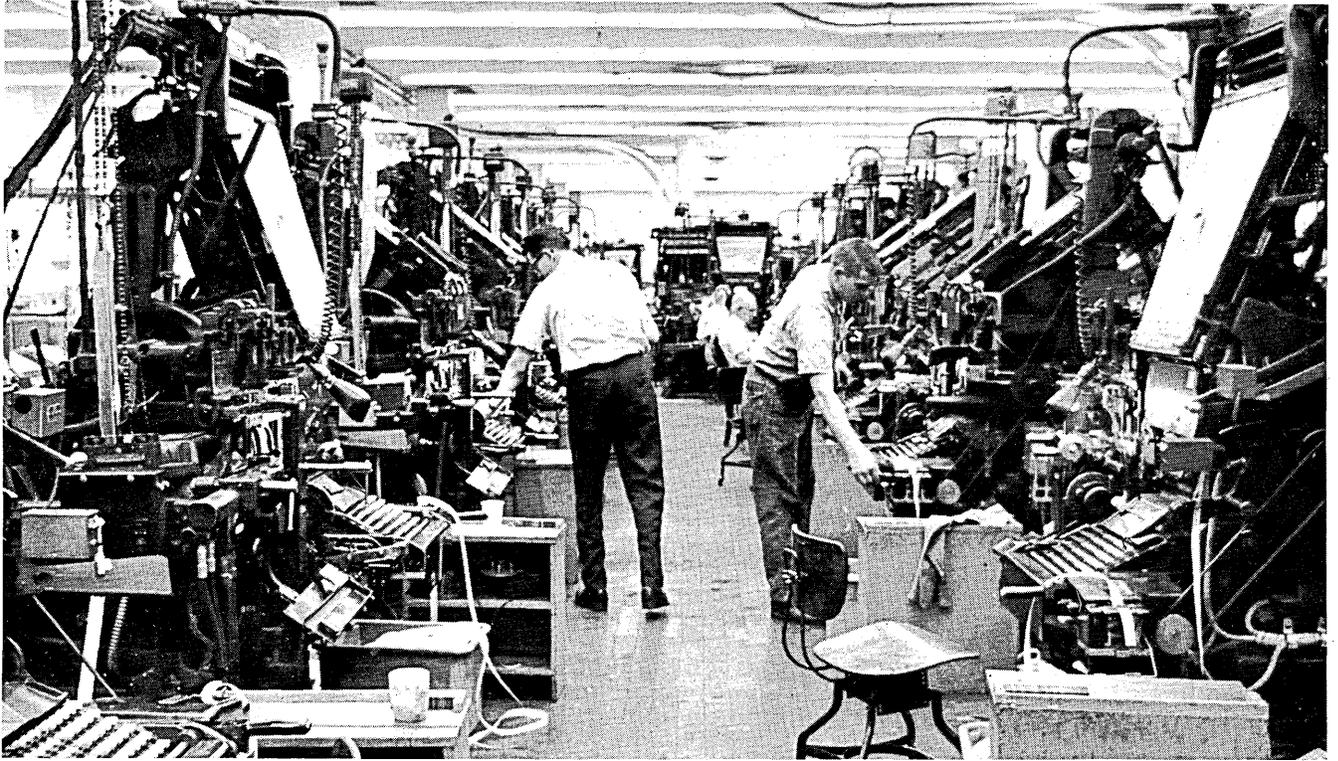
Tape-operated, unmanned linecasters are one result of computerized typesetting as seen at the Los Angeles Times.
