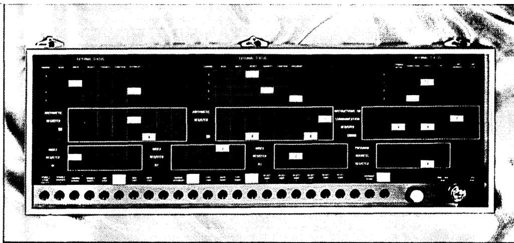
DATA-PANEL indications are visible only when illuminated. Permanently visible legends and grids are provided for operator orientation. Courtesy Control Data Corporation.
