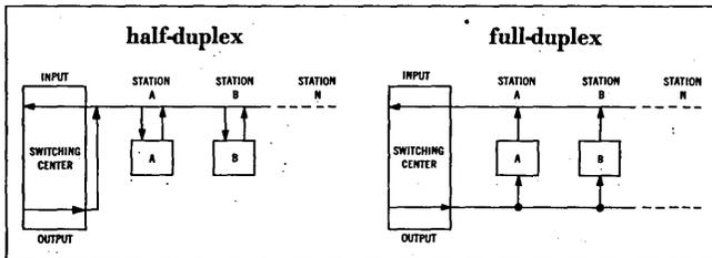
process at any time. With the full duplex circuit all transmit stations are connected to the input side of the switching center and all receive stations are connected to the output side of the switching center. This configuration permits simultaneous input and output traffic from the switching center.
