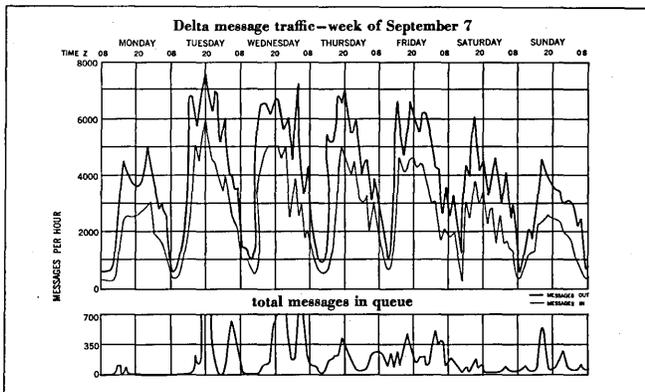
of these systems. The total queuing for each system is relatively low except during peak traffic conditions. The queue buildup is directly related to the traffic distribution. That is, when input traffic arrives and is routed to a given output circuit at a faster rate than transmission can occur over that circuit, a queue will develop for that circuit.
