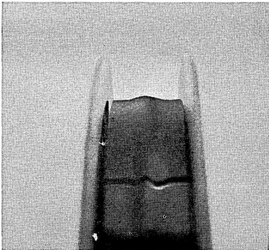
**Complaint.** Semi-permanent ridging and loss of contact caused by microscopic scratches produced in manufacturing or use.
