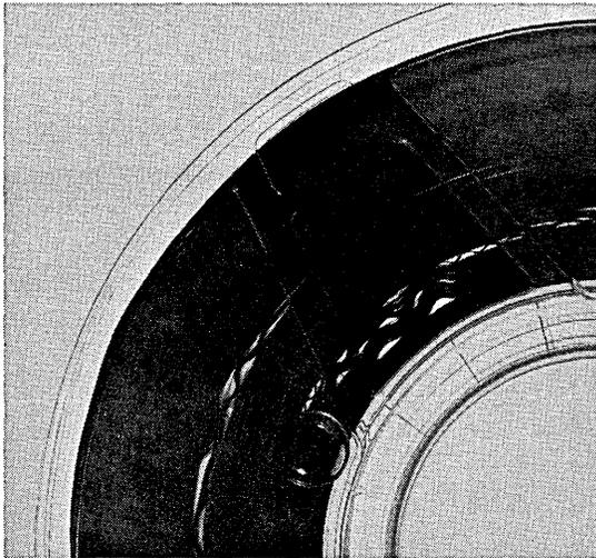
**Complaint.** Cinching during shipping, use or handling results when reel is wound under improper tension or exposed to temperature extremes.
