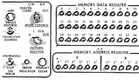
**SELF-TESTING.** RCA MS-1 systems can be supplied with built-in tester to locate read-in and read-out errors.
