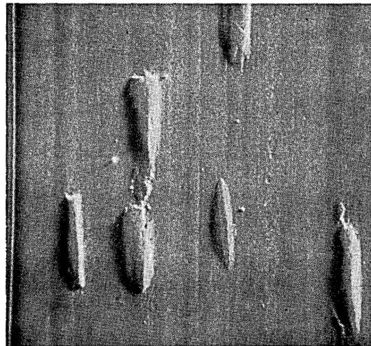
**Complaint.** Dropout-causing clumps of redeposited coating (50X magnification).
