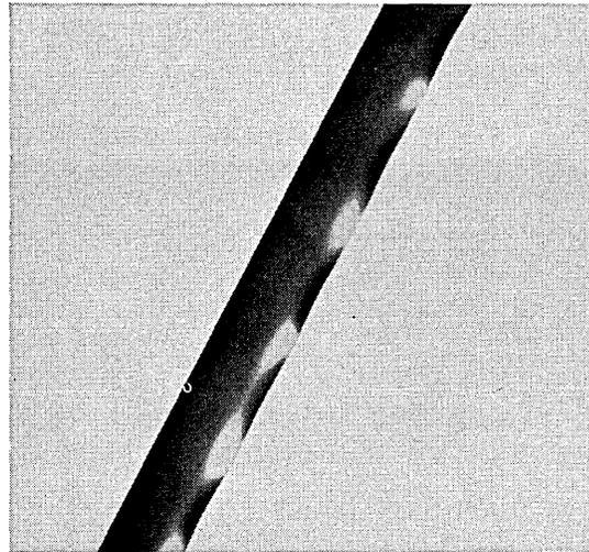
**Complaint.** Wavy edge caused by improper slitting.
