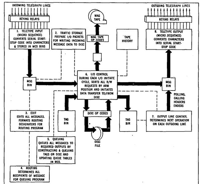
ence of the start bit and code bits. The code bits are assembled into five-bit Baudot characters and packed three characters per computer word. These words are then stored as message segments in bins (typically 32 words) in main core storage. (The assignment of bin locations is handled by a closed subroutine called the available bin program, which allots available bins to all requesting routines. Depending on the system, up to 512 bins are reserved for this function).
