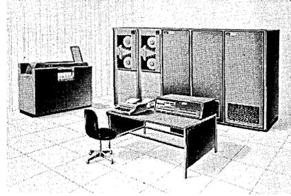
direct memory access channels, standard controller for connection of up to 512 real-time data sources, seven programmable registers, and register-to-register instructions. Software includes a 1620 simulator and FORTRAN II.
