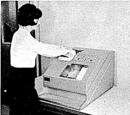
reading rate; its input hopper holds 1,500, and the output holds 1,000. Both are photoelectric units, and have as optional features a 51-column card operation and card reject hopper.
