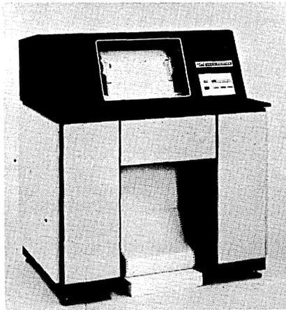
ent characters—numeric, alphanumeric and symbolic—in sets of 48, 64, 96 or 192. It is modular in design, with all electronics on pluggable printed circuit boards, and features dual speed, servo-controlled paper feed. Power requirements are 208/230 volts, single phase, 50 or 60 cycle. The 3550 is supplied in its own soundproofed cabinet, supported by a welded steel frame.
