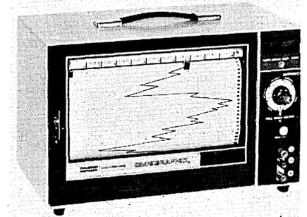
inches/min. Disposable fiber-tipped pens are used on the device to record inputs presented in volts, millivolts, ohms, milliamps, or microamps from
