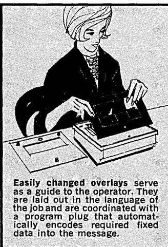
Easily changed overlays serve as a guide to the operator. They are laid out in the language of the job and are coordinated with a program plug that automatically encodes required fixed data into the message.
