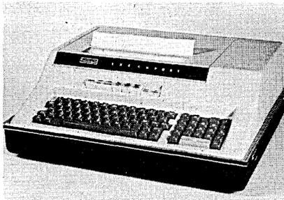
inary telephone lines, the terminal provides 96-character full USASCII capabilities. Its additional 32 characters include symbols and lower case alphabet. Included as integral components are a keyboard; a 10, 15 or 30 cps (operator selectable) thermal page printer; solid-state control logic; built-in telephone coupler and interface; and a universal interface for peripheral accessories. All this and the carrying case weigh less than 30 pounds.
