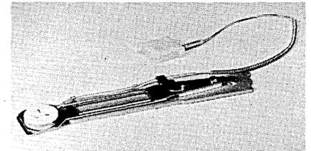
operating with disc packs features a straddle erase design to prevent fringing from a recorded track to an adjacent track. A typical disc drive spindle unit contains 20 head assemblies in a combination of five each of ERW-111501-1, -2, -3, and -4.
