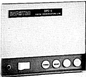
data between a computer and remote peripherals, including printers, card reader/punches, plotters, crt's, etc. The unit includes a logic board and two interface boards. Price is \$1,255, reduced to \$1,060 in quantities of ten. The logic board alone, including all logic and control circuits, is available for \$315. INFOTEC, INC., Rye, N.Y. For information:
