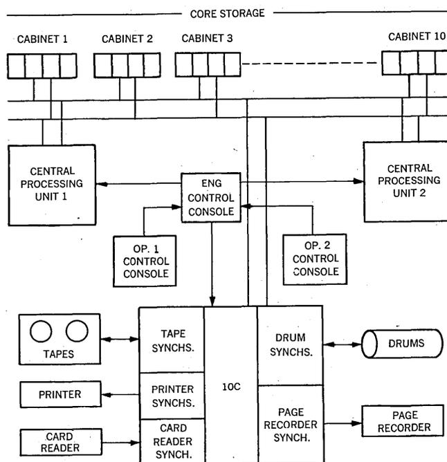
Fig. 1—Block Diagram of a LARC System
