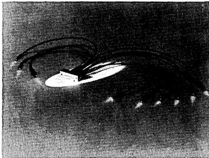
package. One significant advantage of the resulting reader is that the light at any channel can be modulated individually, allowing for accepting coded information on each channel. Price for the fiber optics assembly is under \$50. BENDIX CORP., Sturbridge, Mass. For information:
