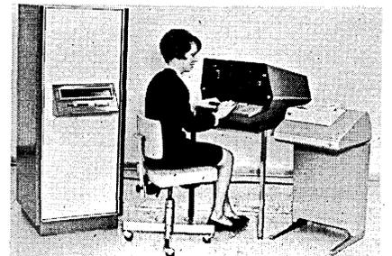
central processor in either parallel or serial mode at transfer rates from 300 to 4800 bps. An IBM-compatible interface adaptor is available; interfaces for other computer systems are available on request.
