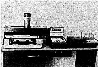
cards. The user can store 10 million bits of information in a cubic foot of space and retrieve or correlate any of this information in two minutes. The system may be linked directly to a computer system and can also serve as a completely independent information retrieval center.
