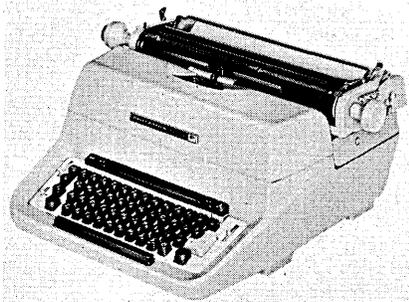
ters using a photoelectric encoding technique. Switch contact unreliability, contact bounce, and RFI/EMI are said to be eliminated. The 720 also protects against operator errors by automatic lockout of the keyboard.
