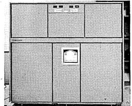
magnetic tape transport and controller and a Honeywell 516 computer. The electronic plotter records information from a crt onto microfilm and/or photographic paper.
