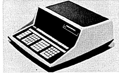
direct and indirect store and recall of data registers enable it to invert a matrix up to 10 X 10. The unit has its mag tape for some I/O, and augments this with provisions for typewriter output. A "learning" mode enables step-by-step program use or checkout. At \$4,900, the price approaches that of a cpu, too. WANG LABORATORIES, INC., Tewksbury, Mass. For information:
