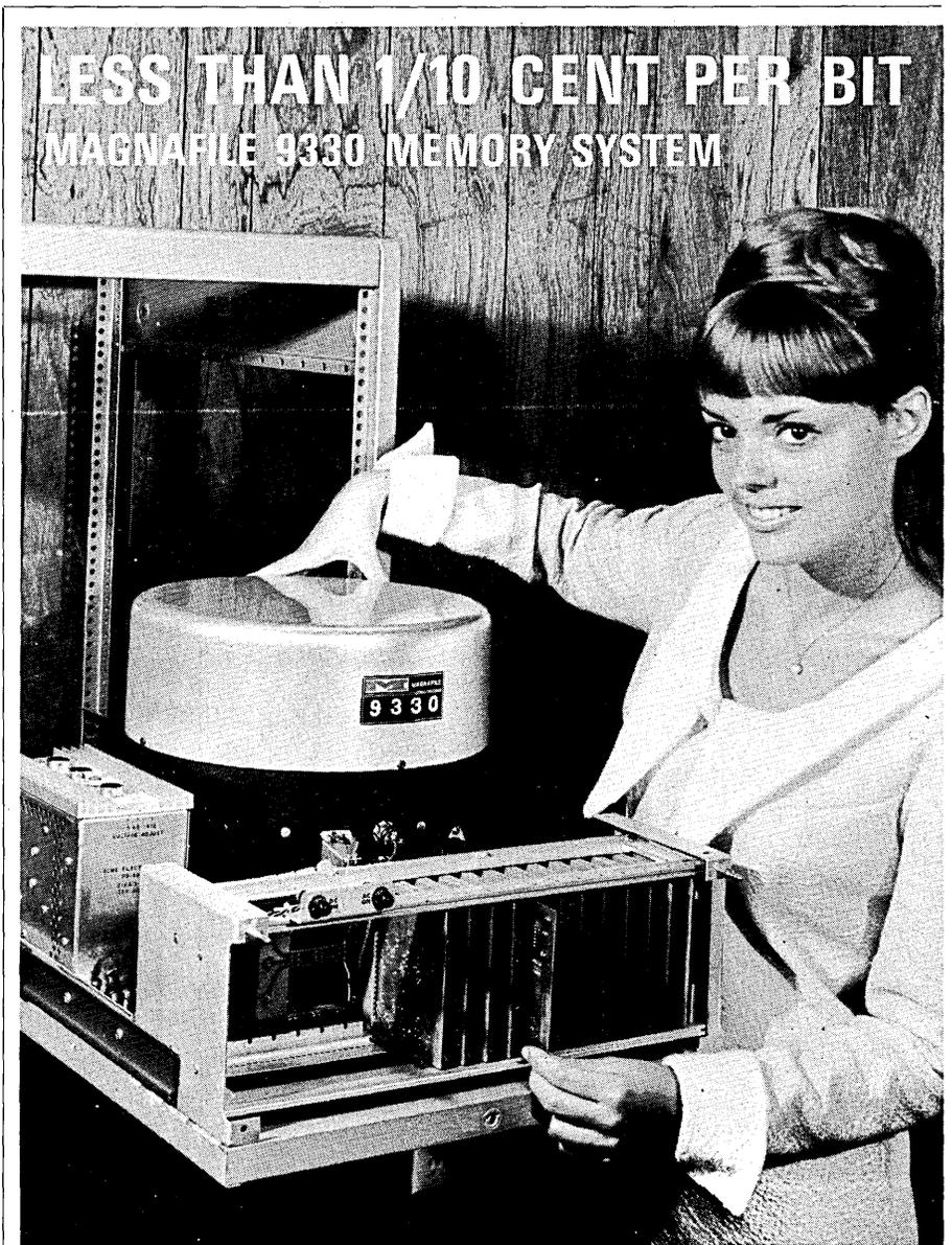
With ten million bit capacity, this new third generation Magnafile memory system paces the field in both economy and reliability. With its head-per-track system, the Magnafile 9330 gives you an average access time of 8.3 or 16.6 milliseconds and the flexibility to meet your application. Write or call for more information — it's credible.
