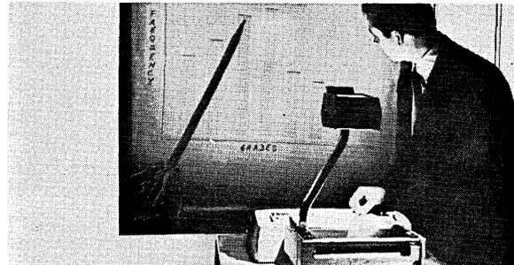
APL 360, the computer language for interactive systems designed by I. P. Sharp Associates Limited, Toronto, Ontario, is displayed here on the 2510T Teleprinter Projector which projects an image up to 144 sq. ft. I. P. Sharp Associates specializes in integrating hardware and software for total computer systems.
