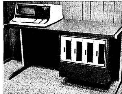
83 msec. The drive architecture features four 256-character buffers corresponding to sectors on the disc, giving a 1024-character addressable buffer, which should aid programming considerations. The diskette drive leases for \$110/month, with maintenance, on a two-year contract.
