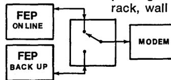
\*T-Bar Universal Fall Back Switches have been used successfully to switch various Front End Processors, including IBM 3705, IBM 270X, UNIVAC 1108, Burroughs 5000, Memorex 1270, DEC PDP-11/45.
