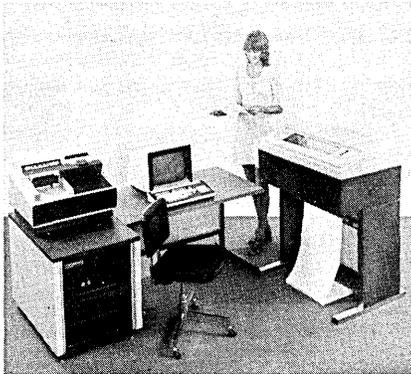
spooling, a standard on the system, makes it possible to input jobs from the 300 or 600 cpm card reader to disc, output another job from the disc to the 300 to 1800 lpm printer, and receive or transmit a third job over a
