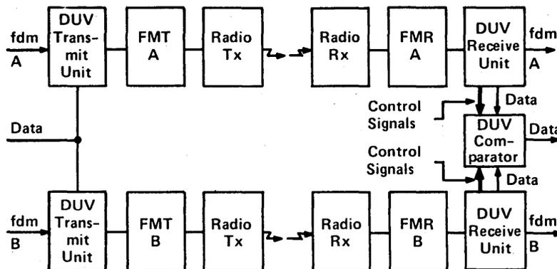
**PARALLEL DUV:** In this one-for-one protection configuration, two frequency division multiplexed signals and one 1.544 Mbps data signal are transmitted over two working radio channels. The comparator equipment then selects from the two decoded bit streams the one that has no bits in error.
