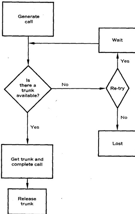
Fig. 2. A simple model of a telephone trunking system is adequate for investigating some call interarrival times, for predicting the number of lost calls, and for analyzing the effects of intermittent line outages.
