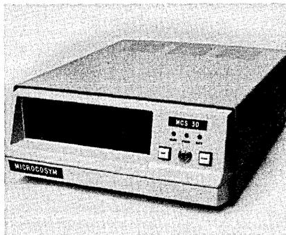
with automatic baud rate detection. Built-in routines are standard and can be accessed remotely. Optional features include additional eight-line modules to a maximum of 32, and expanded memory in 8K or 16K increments to a maximum of 64K bytes. A read-only memory option for program storage eliminates bootloading of the system. A standard eight-line system rents for \$720/month including maintenance on a one-year contract. MICROCOSYM, INC., Peoria, Ariz.
