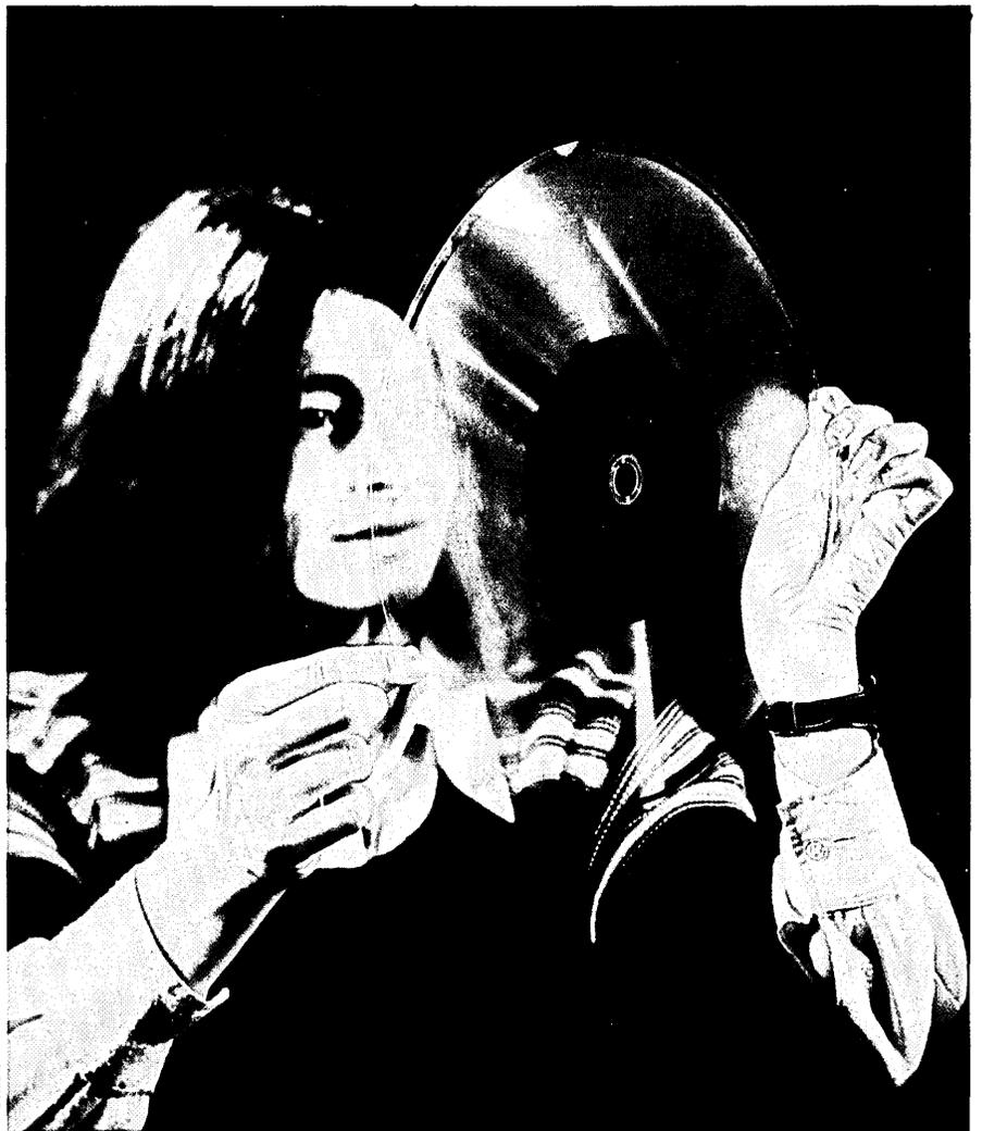
The Thomson-CSF TTV 3620 uses this transparent videodisk. Made of thin glass coated with special resin, the disk is read with a transmissive rather than a reflective optical system. Soon 3M will be manufacturing both kinds of disks.
