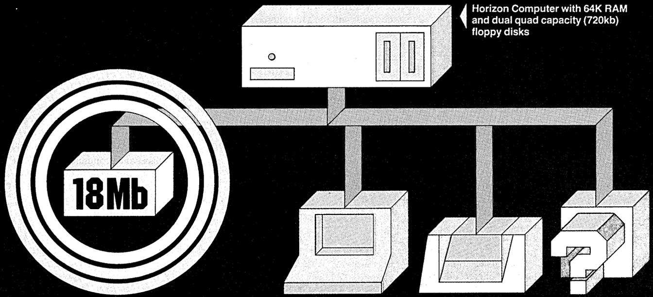
Up to four 18Mb Winchester-type hard disk drives
