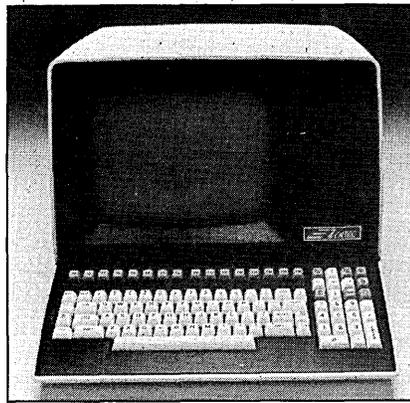
trol keys, 12 special purpose function keys, and 16 programmable function keys. Both RS232 and 20mA current loop interfaces are standard. Communications can be in full- or half-duplex at speeds from 110bps to 19.2Kbps. Production began last month, with volume deliveries expected this quarter. One Zephyr sells for \$1,220; 100 unit price is \$976. ZEPHYR CORP., Santa Clara, Calif.
