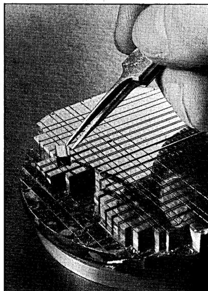
The new thin film heads are like semiconductors and are made by a deposition process. MAGNEX will use a thick wafer and integrate the thin film head with the slider in one piece.
