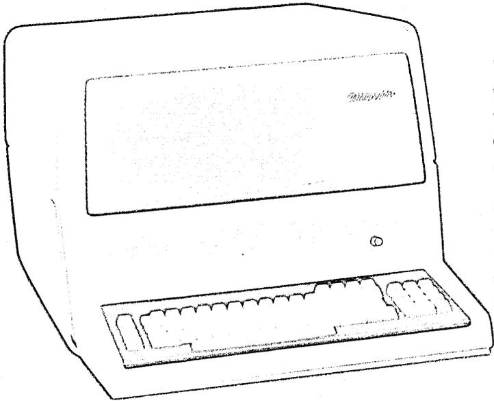
The model 132-1 introduces a new high in 132 column display quality with functional versatility at an economy price. The partial list of features are shown as actually displayed on a 132-1 with the Datagraphix patented Charactron® cathode ray tube.
