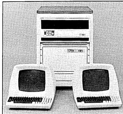
ed for use as modular building blocks in systems for business and industrial applications. The 1/20A is a desktop unit, while the 1/25A is a rack-mountable unit. The two general-purpose, ready-to-run systems are the desktop MCZ-1/50 and the rack-mounted MCZ-1/70. All four use the vendor's Z80 microprocessor with 64KB of memory, and each sports interrupt-driven console capability and a floppy disk con-
