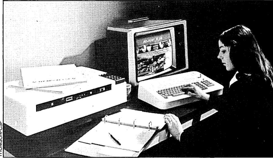
The Thomson-CSF 3620 being used with a microcomputer for self-paced instruction. The small keypad in the lower righthand corner of the machine is used for random access to a video frame.
