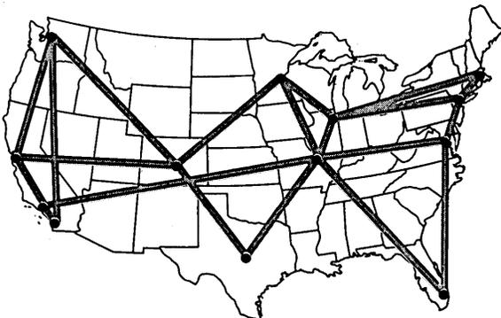
Conventional fixed network is difficult and expensive to expand and modify as needs grow. And they always do. Communication and utilization of data base records from twice removed nodes is prohibitively expensive in applications programming, so more lines are the only viable solution. And that is expensive, too.
