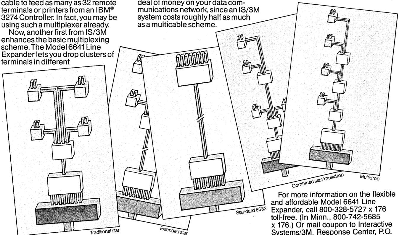
Model 6641 Line Expanders direct data from an IS/3M 6632 Multiplexer attached to the IBM 3274 Controller to one, two, three, or four IS/3M 6600 Multiplexers that can be arranged in a variety of network
