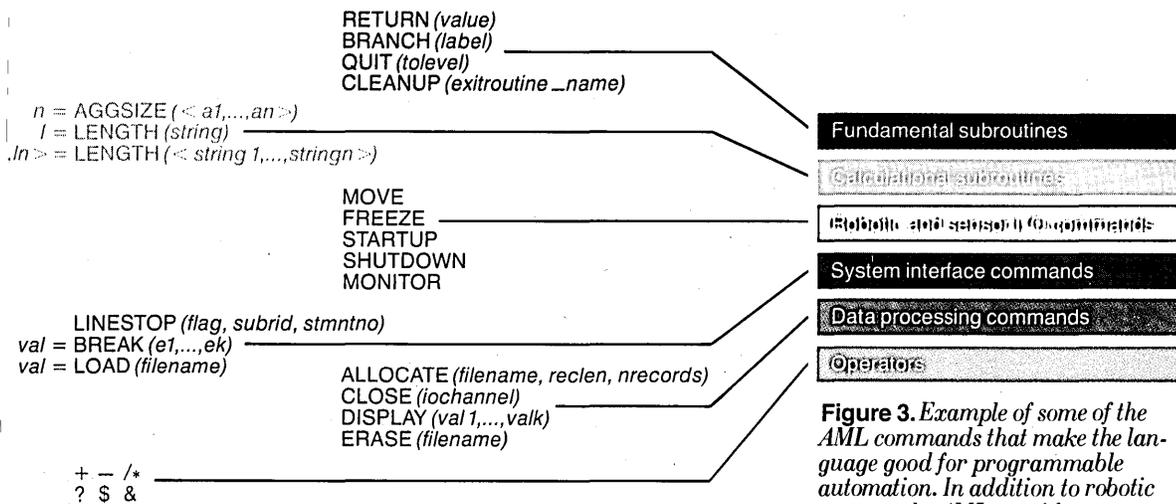
**Figure 3.** Example of some of the AML commands that make the language good for programmable automation. In addition to robotic commands, AML provides an abundance of communications and data processing commands.
