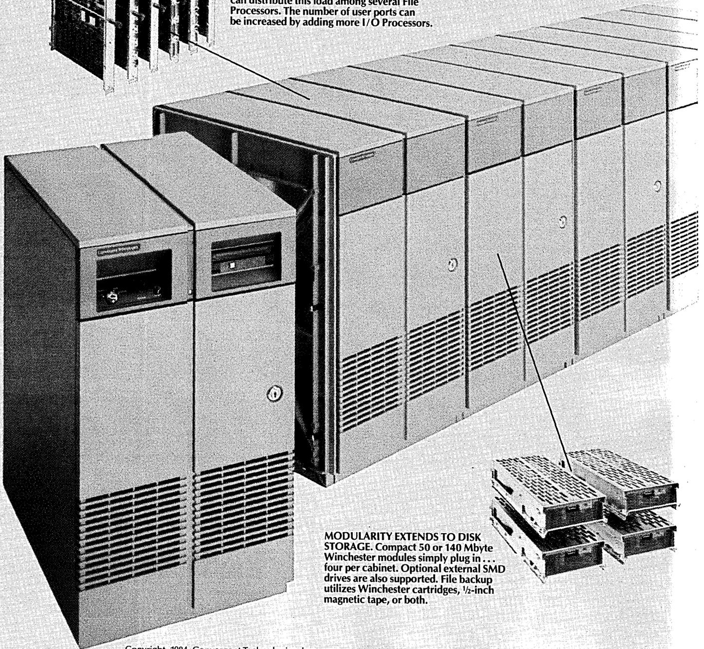
**MODULARITY EXTENDS TO DISK STORAGE.** Compact 50 or 140 Mbyte Winchester modules simply plug in . . . four per cabinet. Optional external SMD drives are also supported. File backup utilizes Winchester cartridges, 1/2-inch magnetic tape, or both.
