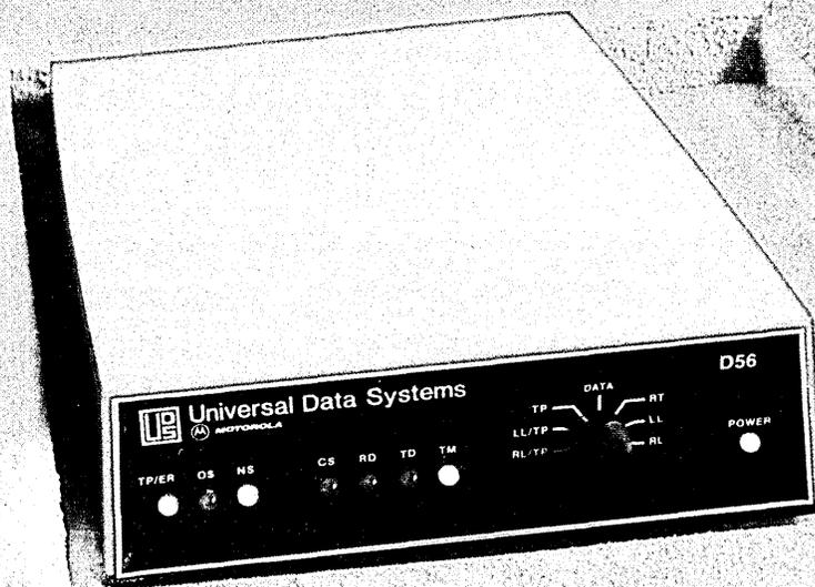
Large-scale integration has arrived in DSU/CSU design! The result: 54% less volume and a 40% cut in power consumption for Universal Data Systems' latest units. DSU and CSU are combined on a single printed circuit board. Data rates of 56 kbps (CCITT V.35) or 9.6 kbps (RS-232C) are available.
