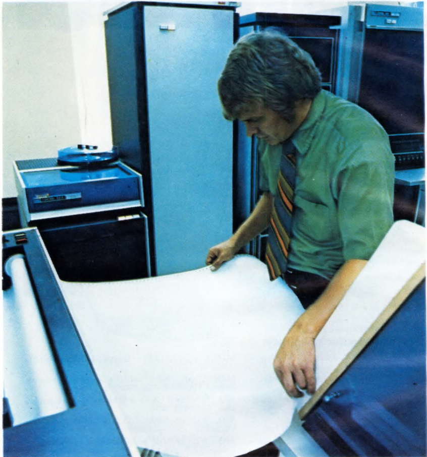
X-Y plot shows position of cells and interconnection scheme. In the background is the main computer, a CDC 1700, a disk system with 1.5 million word capacity, and DEC PDP 11/15 used as an I/O processor and plotter control.
