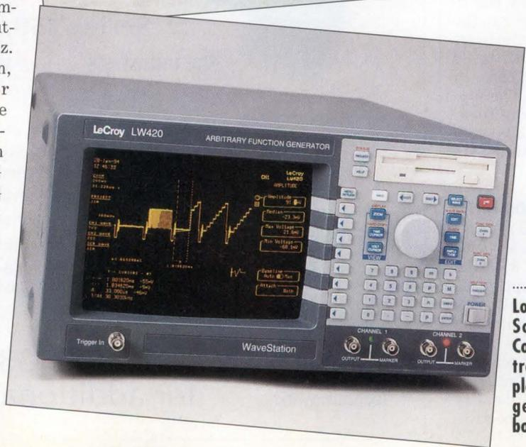
Looking exactly like the vendor's Scopestation 140 DSO, LeCroy Corp's LW420 and 410 output arbitrary waveforms at 400M samples/sec. Like the Scopestation, the generators include PC motherboards.
