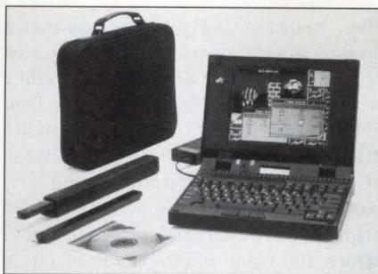
**No, it's not a workstation, it's a logic analyzer. Tektronix's 100-channel TLA 510 (\$18,000) and 200-channel TLA 520 (\$33,000) perform state analysis to 100 MHz and timing analysis to 400 MHz.**
