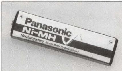
cylindrical cells. The cells measure 17 mm long×6.1 mm wide×67 mm high. The cells have a nominal output voltage of 1.2V and a nominal capacity of 760 mAh. \$8 (500 to 1000). **Panasonic Industrial Co.**, Secaucus, NJ. (800) 848-3979. **Circle No. 432**
