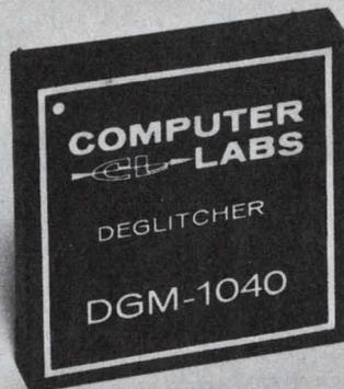
Computer Labs introduces a new line of modular deglitchers with the DGM-1040 & DGM-1080. Used to eliminate the non-linear effects of glitches in the output of D/A Converters, these miniature modules generate an output signal with extremely high spectral purity, required for TV signal reproduction, CRT displays, and waveform generation. Acquisition times as low as 15 ns and linearity of 0.01% make these the highest speed and most versatile deglitchers available commercially.
