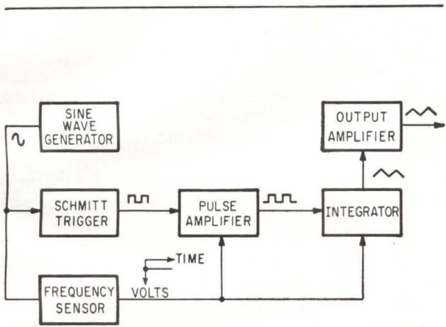
TRIANGULAR-WAVE generator uses a frequency sensing circuit to keep amplitude constant—Fig. 1
