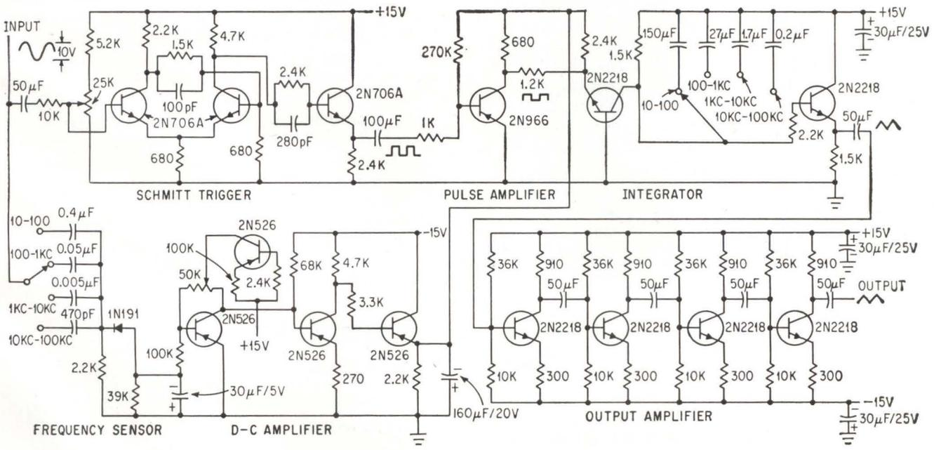
CIRCUIT of the triangular-wave generator uses 14 transistors—Fig. 2
