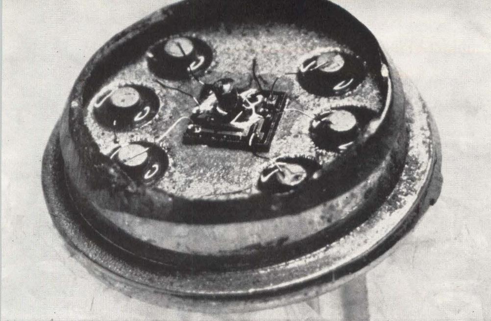
EXPERIMENTAL INTEGRATED sensing circuit constructed at Raytheon incorporates a piezo-junction accelerometer. Preliminary measurements indicate sensitivities of the order of 300 microvolts per g with a seismic mass of 0.1 gram. Work was described by W. Rindner, R. Wonson and G. Doering at the Solid-State Circuits Conference
