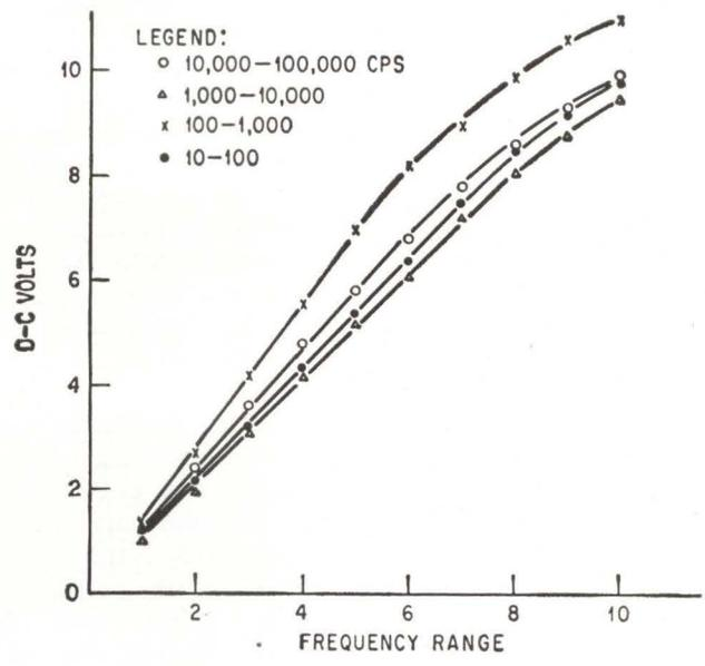
OUTPUT VOLTAGE of the frequency sensor is linear, except at the upper frequency range—Fig. 3
