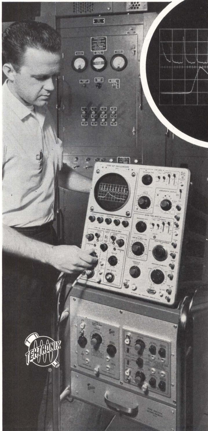
Dual-trace display shows the lower trace as an expanded presentation of the intensified portion of the upper trace. Note the bright display of small spot size and uniform focus over the full viewing area.
