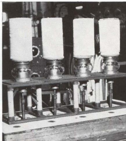
**SPECIAL JACKETS** are used for thorough anode outgassing during exhaust of ML-6697 (F.A.C.). Other unusual methods have been developed for oven baking, anode heating, grid outgassing, and cold cathode desparking.
