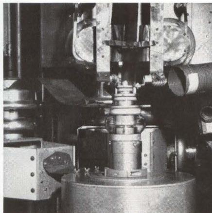
**UNIQUE 1.2 MW TEST SET** is used for high-power rf amplifier test of water-cooled ML-6696. Tests are programmed from remote control console.
