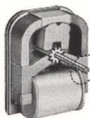
This cutaway view of the Cyclonome Stepping Motor reveals its unique simplicity. Its only moving part is a rotor without windings, without brushes. The precise, incremental rotation of the rotor is due solely to magnetic force. For a
