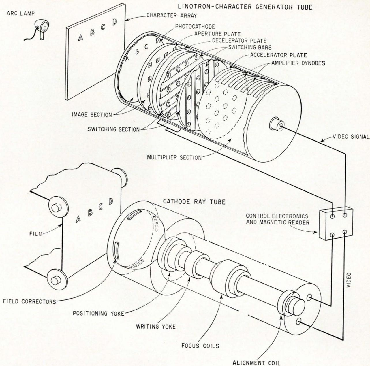
**Character generator's** switching section selects one of the 256 video signals representing the characters that have been projected on the tube's photocathode. The video signal is then sent to the cathode-ray tube where it sweeps out the character in its proper position on the page to be printed. The characters expose film which is developed off-line and used to make printing plates.
