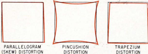
PARALLELOGRAM (SKEW) DISTORTION
