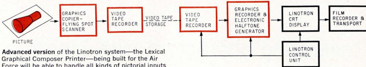
**Advanced version** of the Linotron system—the Lexical Graphical Composer Printer—being built for the Air Force will be able to handle all kinds of pictorial inputs with the additional subsystems shown in color.
