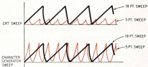
**Sweep slopes** on the crt must be the same for all type sizes so phosphor brightness won't vary. Sweep slope in the Linotron tube becomes steeper as the point size gets smaller because the crt determines sweep time. The Linotron's sweep amplitude remains constant.
