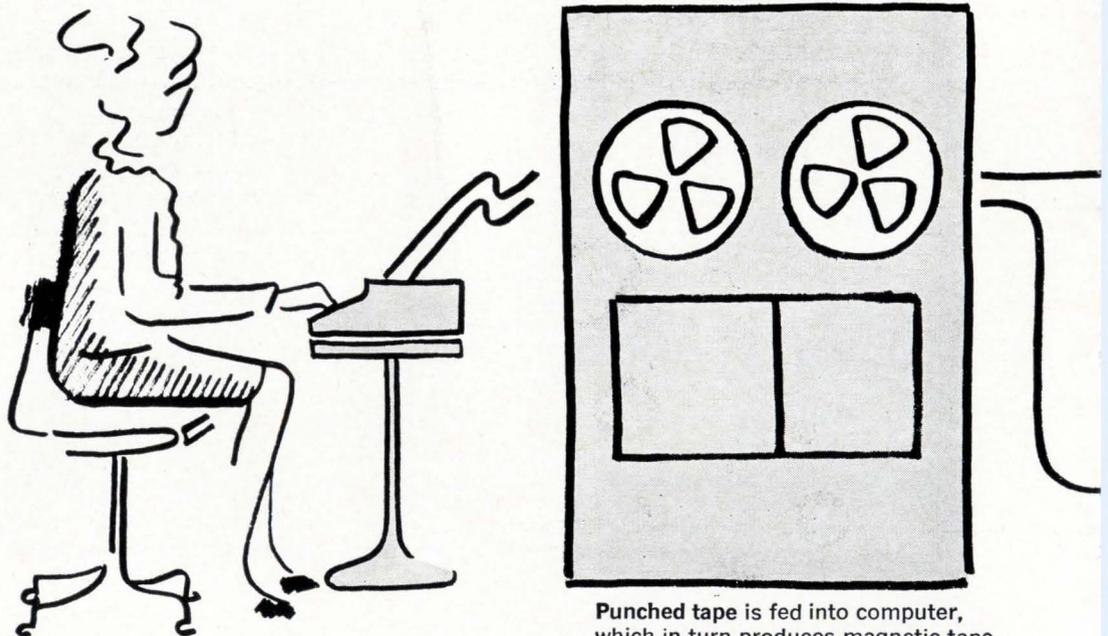
Punched tape is fed into computer, which in turn produces magnetic tape.
