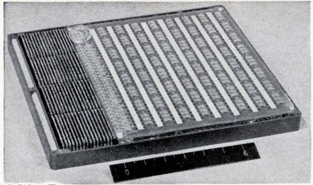
In partly assembled braid memory, above, a large printed-circuit board carrying the sense circuits in flatpacks is installed on top of the braid. The U-shaped cores will be inserted through holes in the p-c board. Adding the drive circuits increases the thickness shown here by about 50%. Complete assembly of braid memory in exploded form, at left, shows drive circuits on the bottom, cores and braid in the middle, and sense circuits on top.
