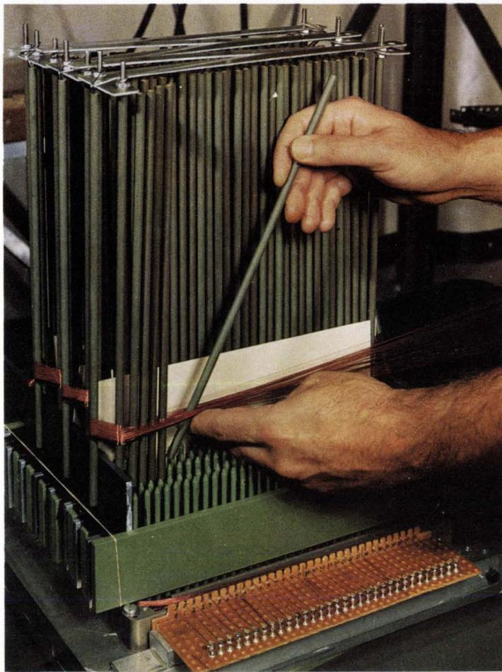
As the separator is moved toward the workpiece, the operator twists it into a vertical position. He must be careful not to lose the separation of the wires during this step. He then sets the separator — a hollow tube — onto one of the Teflon-covered nails at the workpiece.
