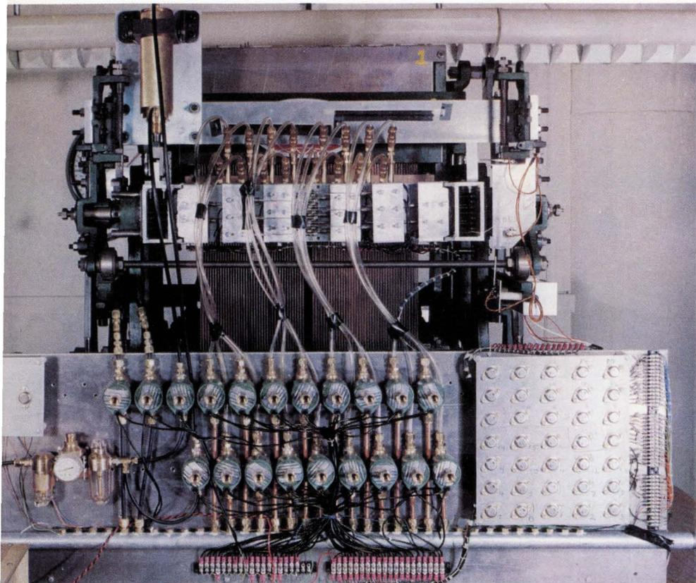
**Tape-controlled block**, at the upper end of the clear plastic hoses, contains free pins which, with the block lowered, fall to the rear of the block. When the block is in its raised position, shown here, air jets set the pins to establish the combination of wires to be separated during the lift's next move, following immediately.
