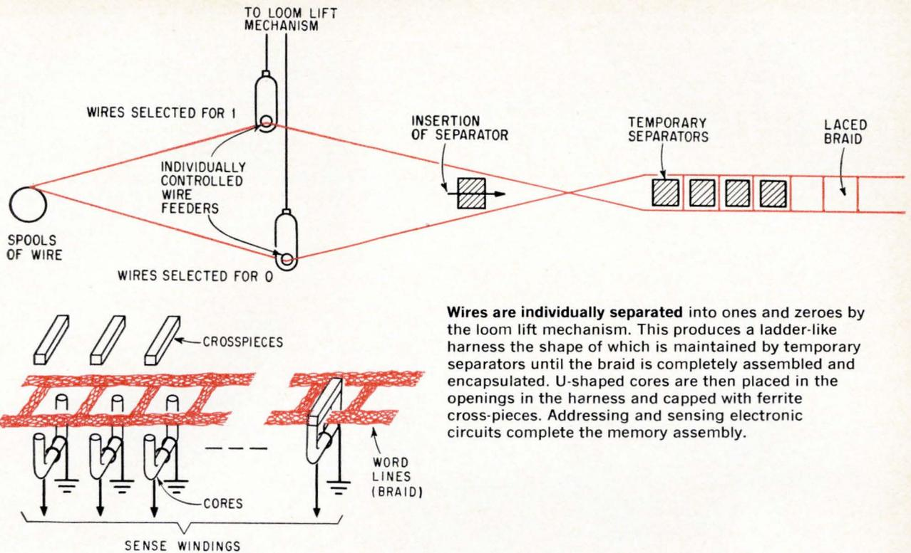
**Wires are individually separated** into ones and zeroes by the loom lift mechanism. This produces a ladder-like harness the shape of which is maintained by temporary separators until the braid is completely assembled and encapsulated. U-shaped cores are then placed in the openings in the harness and capped with ferrite cross-pieces. Addressing and sensing electronic circuits complete the memory assembly.
