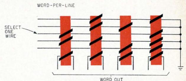
Word-per-line organization is basis of braid memory. The wires making up the braid are word lines. They couple a signal to sense lines by way of the cores.
