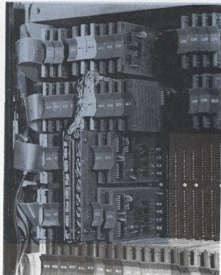
**Before and after.** The big black box is the memory assembly for the old PDP-8. The small assembly above stores just as much data and makes it accessible just as fast.
