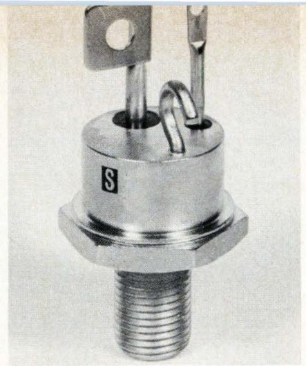
trols and power supplies. Specifications include a typical  $f_t$  of 15 MHz, saturation voltage of 1.0 v maximum, and a power dissipation of 300 w at 100°C.
