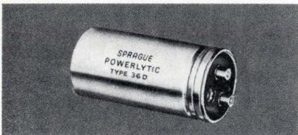
**TYPE 36D POWERLYTIC® CAPACITORS.** For use in computer power supplies, control equipment, energy storage, etc. Low impedance construction. Up to 650,000  $\mu$ F at 3 V. Ratings from 3 to 450 V. Can be operated at 85°C. Tapped 10-32 terminals simplify filter bank assembly. Write for Engineering Bulletin 3431C or;
