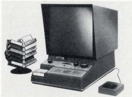
trieve COM data recorded in cine or comic format or be used as a general-purpose 16-mm microfilm display. It accepts 100-foot rolls of microfilm loaded in Quantor or 3M cartridges. Each cartridge stores up
