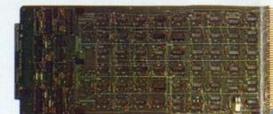
**I/O Distributor.** Model 14629-XX. In conjunction with Intelligent Cables (see text), the I/O Distributor provides up to eight interfaces—serial or parallel in any mix. Small version accommodates four interfaces. A DMA version allows data transfer rates up to 250K bytes per second.
