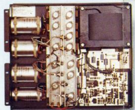
**Standard Power Supply.** Model 12044-00. Supplies +5V @ 25 Amps, +12V @ 4 Amps and -12V @ 9 Amps.
