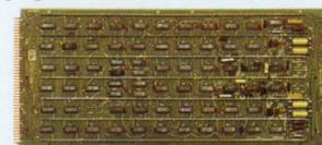
**EIA RS232 Interface.** Model 14236-5X. For one CRT at baud rates from 110 to 9600. Half-duplex operations only.
