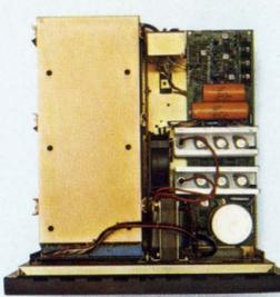
**Alpha LSI-3/05 B, NAKED MILLI Series.** Model 10375-XX. Includes LSI-3/05 CPU (Type 1) described at left, plus 5 half-card chassis with fan, 15-Amp power supply and Operator's Console. Full memory options.
