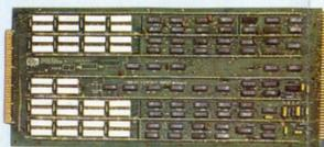
**32-bit Relay Input Module.** Model 13215-00. Operates as one 32-bit, two 16-bit, or four 8-bit inputs.
