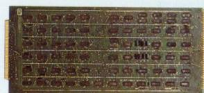
**64-bit Input Module.** Model 13219-00. Provides 64, 32, 16 or 8-bit inputs with individual strobes.
