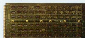
**Automatic Calling Unit (ACU) Multiplexer.** Model 13523-0X. Provides interfaces for one to four Model 801 ACU's, or equivalent. Simultaneous operations, full digit buffering and sense date-line busy. Four vectored interrupts per ACU. Available for either two or four ACU's.
