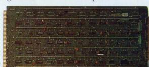
**I/O Driver Module.** Model 13222-00. Units drive the computer I/O bus up to 25 feet, buffer internal I/O bus from external noise. Does not include memory signals.
