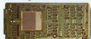
**Half-card Core Memory.** Model 11671-XX. 4K words. For either NAKED MILLI/ALPHA LSI-3/05 or NAKED MINI/ALPHA LSI-2 Series Computers.
