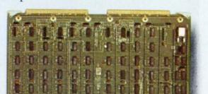
**Dual CRT Interface.** Model 14236-1X. For two CRT's or leased line modems. EIA RS232 interface with two half-duplex channels, each with one output control line and one input status line. Baud rates from 110 to 9600.
