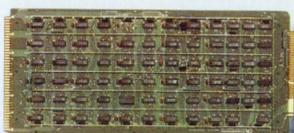
**16-bit Digital Input/Output Module.** Model 13213-00. Provides input and output registers which may be used as one 16-bit or two 8-bit registers. DTL/TTL compatible.
