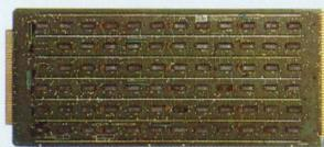
**Paper Peripheral Controller.** Model 14223-00. Single device controller for paper tape reader, paper tape punch, line printer or card reader. Cabling separate.
