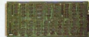
**NAKED MILLI LSI-3/05 CPU, Type 0.** Model 10300-00. Small low-cost processor offers exceptional power and features. 95 instructions, Power Fail Restart, vectored priority interrupts and 16-bit DMA port.
