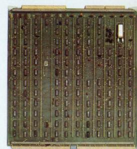
**Magnetic Tape Controller.** Model 14224-00. Provides interfaces for one to four 9-track standard tape units, or equivalent. Cabling separate.
