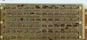
**Moving Head Disk Controller.** Model 14530-XX. Provides interfaces for one to four standard moving head disk drives, or equivalent. 1500 or 2400 RPM. Cabling separate.
