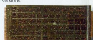
**16-channel Priority Interrupt Module.** Model 13220-00. 16 interrupts with acknowledgement lines.
