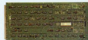
**Synchronous Modem Controller.** Model 14513-00. Double buffered, half or full-duplex interface for synchronous communications line (point-to-point, multipoint, or direct dial). EIA RS232C/CCITT compatible, programmable synchronous character, and one special character detect. Odd, even or no parity and 5-8 bit frame size program selectable. Transfer to 9600 baud.
