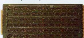
**Utility I/O Interface Module.** Model 14223-00. General purpose interface with 8 or 12-bit output transfers with 4 control bits in parallel.
