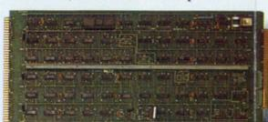
**Asynchronous Modem Controller.** Model 14535-0X. For one asynchronous line (point-to-point, multipoint, or direct dial). Fully programmable for mode, character size, parity, echoplex, diagnostic loop-back, special character detect, variable stop bits. Send/receive speed individually selectable with jumpers—75 to 9600 baud. Available as EIA Interface with full Data Set Controls or as Current Loop Interface.
