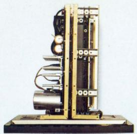
**Alpha LSI-3/05, NAKED MILLI Series.** Model 10373-XX. Includes LSI-3/05 CPU (Type 1), with LSI Family compatibility, three half-card chassis, 10-Amp power supply and Operator's Console. This small, low-cost computer offers exceptional power and features, including 95 instructions, Power Fail Restart, vectored priority interrupts, Real-Time Clock, AutoLoad capability and 16-bit DMA port. Full memory options.
