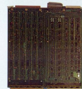
**NAKED MINI LSI-2/20 CPU.** Model 10400-00. Designed for high-performance applications. Twice the performance of the LSI-2/10 for only a nominal increase in cost. Also includes Power Fail Restart.
