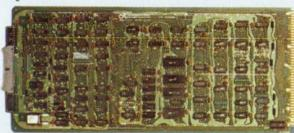
**Floppy Disk Controller.** Model 14566-01. Provides interfaces for one to four IBM-compatible standard floppy disks, or equivalent. Cabling separate.
