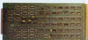
**32-bit Relay Output Module.** Model 13214-20. Operates as one 32-bit, two 16-bit, or four 8-bit outputs.
