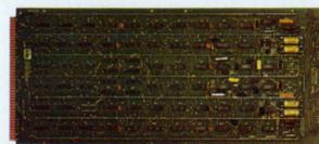
**Dual TTY Interface.** Model 14236-21. For two modified ASR-33 Teletypes. 20 mA Current loop, 110 baud, two half-duplex channels. Has circuit for programmed motor on/off.
