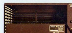
**Power supplies for LSI-3/05.** Model 12046-0X. Open frame power supplies mount in any plane. Supply +5V @ 10 Amps, +12V @ 0.8 Amps, -12V @ 0.8 Amps; +12V @ 1 Amp, -12V @ 1.5 Amps. With fan.
