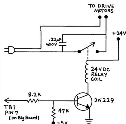
The -5V provides a reverse bias for the transistor so it turns off. The relay is a Guardian IR-1225-2C-24D.
