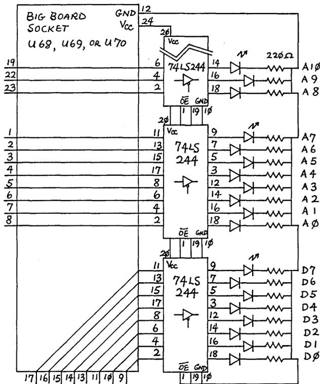
Mini Front Panel Z80 Socket Connection
