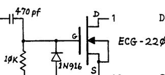
Figure 2 - Big Board II Floppy Interface Modification
