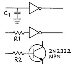
Figure 2 - Controlling Frequency Response
