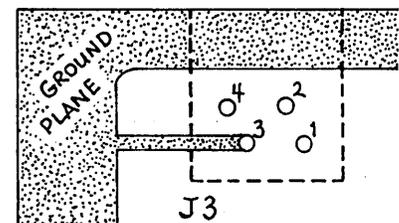
Gently scrape the green solder mask from the ground plane (large copper area) so you'll have a space to solder the capacitor leads. Keep the capacitor leads very short.
