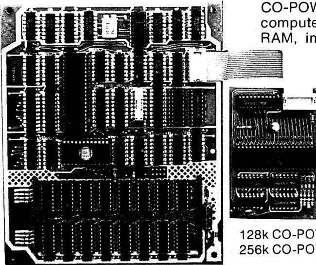
CO-POWER-88 is a 16-bit 8088 coprocessor for Z80 CP/M computers. Both versions of CO-POWER-88, 128k and 256k RAM, include both CP/M-86 and MSDOS, complete with IBM-PC compatibility. A facility for transferring data files between CP/M and MSDOS is included.
