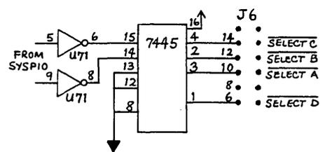
Figure 2 - Select Circuit to Access 4 Drives with Pro-8+
