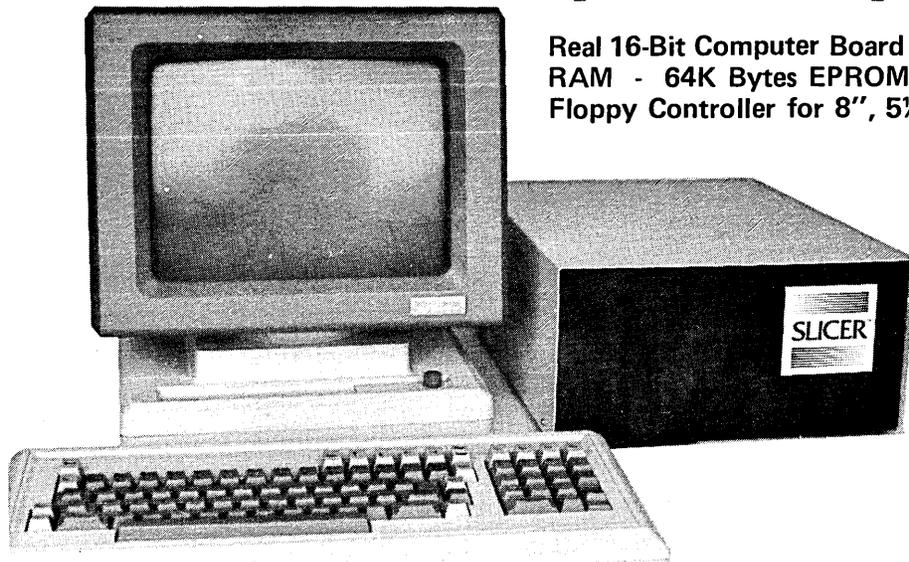
Real 16-Bit Computer Board with 80186, 256K Bytes RAM - 64K Bytes EPROM, Two RS232C Ports and Floppy Controller for 8", 5¼" and 3½".
