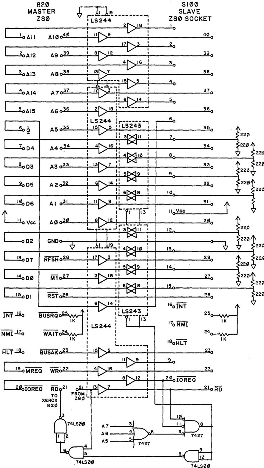
Editor's Note: The  $\overline{RD}$  qualification circuit doesn't appear to qualify the  $\overline{RD}$  signal to Xerox 820's pin 21. However, Jim double checked the original circuit against the schematic and says that this is the circuit that is working.
