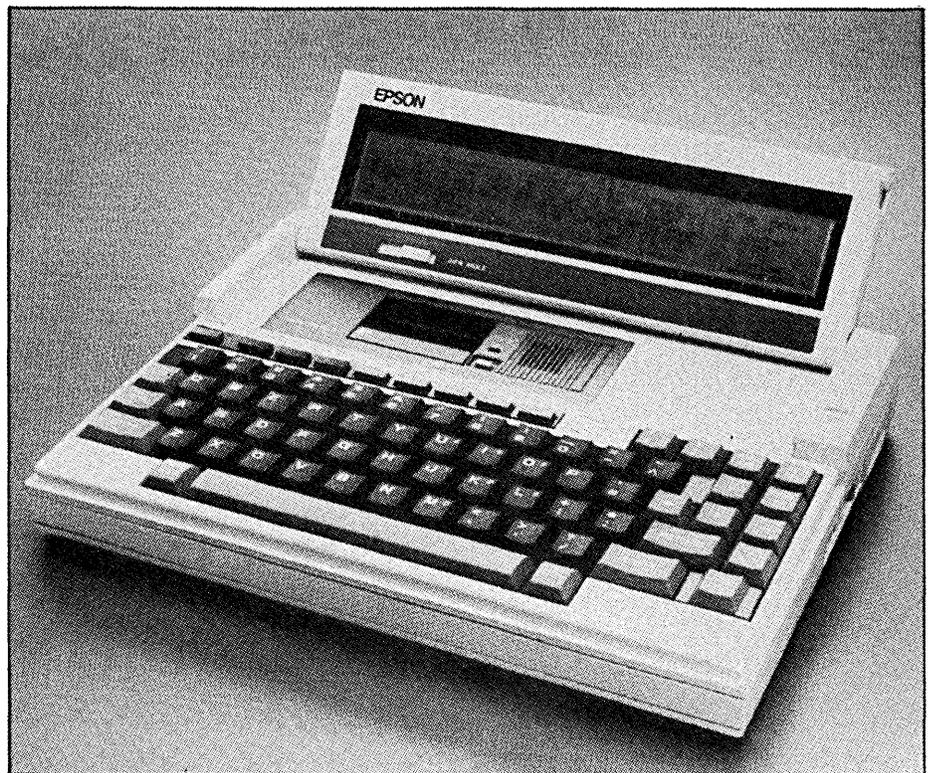
Epson PX-8 Geneva: 8-line by 80-character display, built-in microcassette, WordStar, and CP/M.
