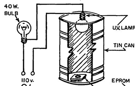
bottom of the can, and insert the bulb down into the can until it is about 1/2" above the EPROM's window. A 20-min-
