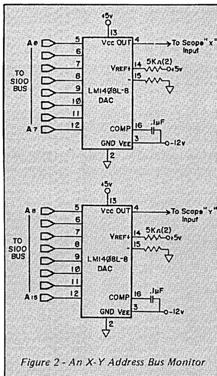
Figure 2 - An X-Y Address Bus Monitor
