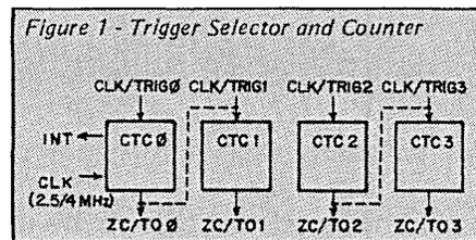
Each of the channels consists of a trigger selector and a resettable counter (see Figure 1). The trigger preselector sends a "decrement" signal to the counter, which keeps track of the count and generates any output signals. The trigger selector is detailed in Figure 2, showing the multiplexer (which selects between the CLK/TRIG or pre-scaler inputs) and the pre-scaler types (divide by either 16 or 256).
