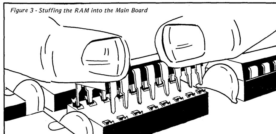
Figure 3 - Stuffing the RAM into the Main Board
