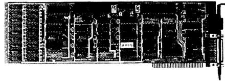
Z-80 single board slave processor that runs CP/M applications on a PC and is compatible with the TurboDOS multi-user operating system.
