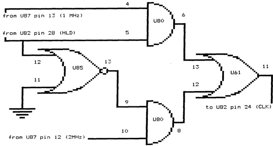
multiplexer, using leftover gates on your Kaypro circuit board. You'll need to cut six traces and then add eight wires. You won't need to bend out any with this method. The trace cutting requires precision and dexterity; read before attempting. See Figure 2.
