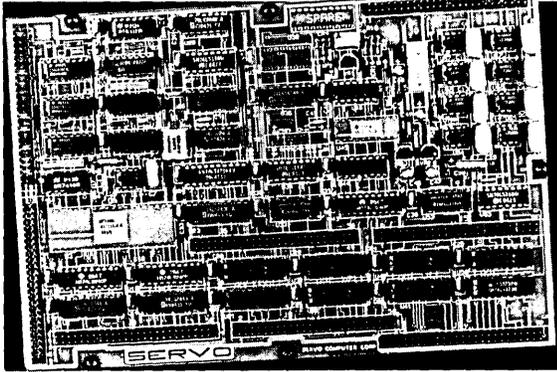
The Servo Process Control Board is a general purpose multi-channel analog and digital input/output controller which can communicate with and control most medium-scale industrial processes. Designed to work with the Servo Industrial Microcomputer, (or other computers which support the SASI Interface), it offers great accuracy at prices starting as low as \$495.
