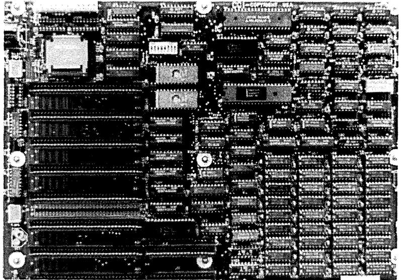
The Challenger XT-186 offers full IBM PC-XT compatibility. It supports industry standard operating systems: MS-DOS, PC-DOS, 1.0 through 3.1, CP/M and runs all existing software with higher performance. The XT-186 mother board can directly replace any existing PC or PC-XT mother board, as it has the same physical dimensions and mounting holes. The Intel 80186 and 640K on-board 16 bit path RAM makes the XT-186 the fastest PC currently available.
