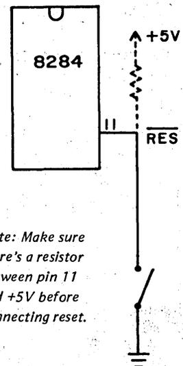
Note: Make sure there's a resistor between pin 11 and +5V before connecting reset.
