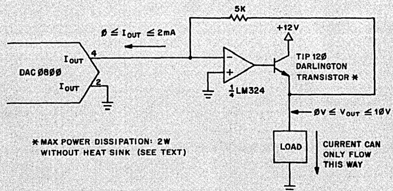
Figure 3A - Connecting A DAC To A Speaker
