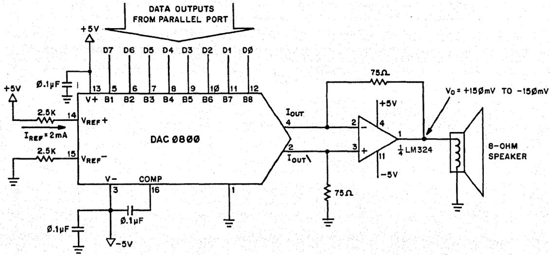
Figure 3B - Outputting A Byte Of "Ones"
