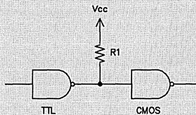
Normally, TTL logic 1 voltage is not enough to drive CMOS inputs, but a pull-up resistor (R1) can be used to bump the level up to what CMOS expects.
