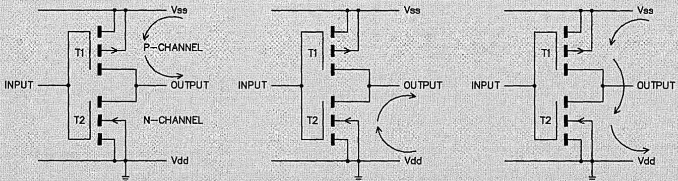
**A** Low inputs cause T1 to conduct so the output is +5v.
