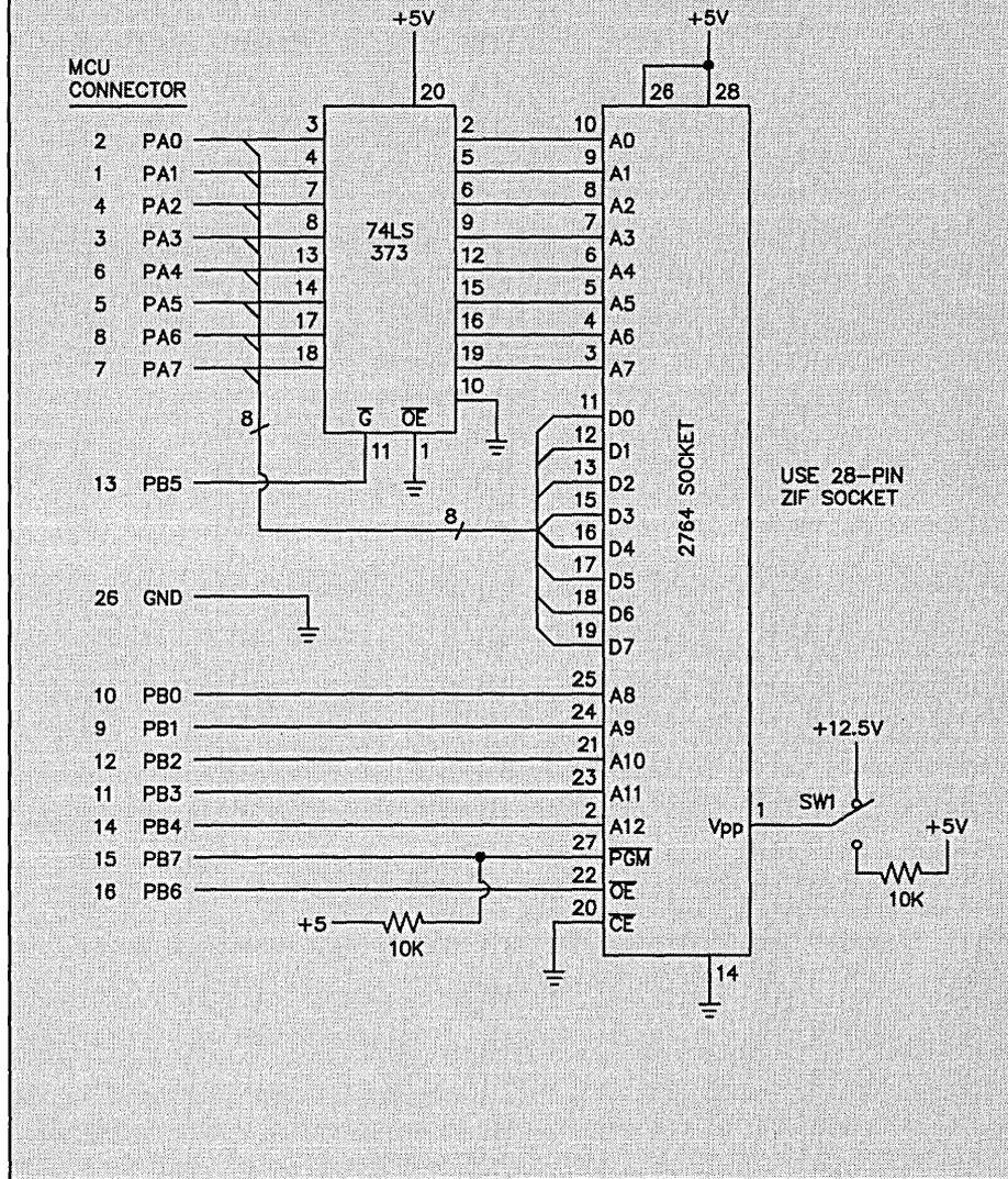
normal 28-pin sockets. Solder one into the board, then plug the other into the top of the soldered one. When the top socket wears out, just replace it. The sockets with the round, machined pins work best for this.
