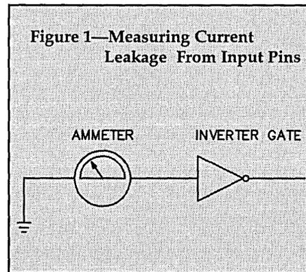
Part of the reason chips draw static current is that transistors aren't perfect. (Many of us have this problem). Theoretically, transistors are switches that turn on and off. In reality (oh no, not that), transistors are slightly on even when they're off.
