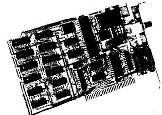
Based on the TRW THC10681 hybrid flash converter, its high signal-to-noise ratio yields excellent accuracy at the Nyquist limit.
