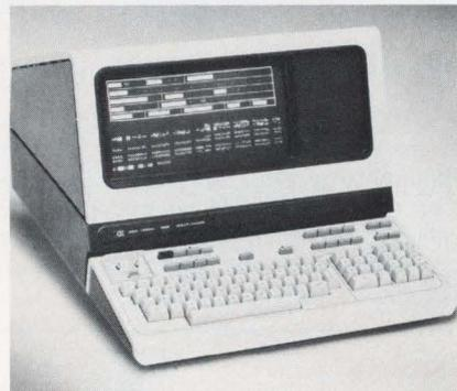
channel protocol for half-duplex operation. The CRT also has a new keyboard layout and includes absolute and relative cursor sensing and positioning.
