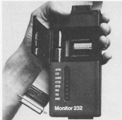
in the echo mode. The unit continuously displays DRT, CD, DSR, CTS, RTS, RD, TD, and TEST INDICATOR on eight LEDs. Pin connections are available for oscilloscope monitoring. Power comes from the line, batteries or rechargeable batteries.
