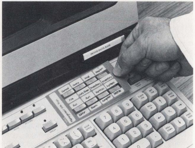
**User-defined management information keys on the Image/1000 data base systems enable users to load or compile a program, query the data base, or monitor the status of multiple tasks.**
