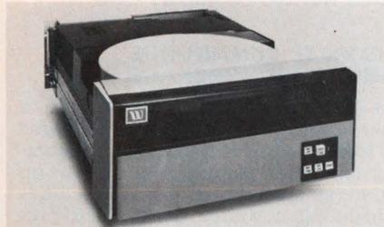
tridges, provides up to 2200 bpi. Wangco reduced the vertical rack space to 7-3/4 inches with its new "side throw" voice coil positioning system. The new light weight magnesium positioner also speeds access time. Drive prices range from \$3100 to \$4470. *Wangco Inc., Los Angeles, CA.*
