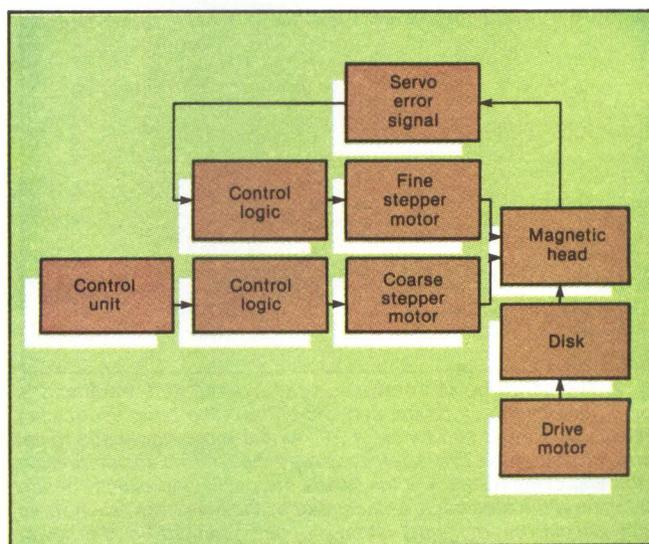
**Fig. 1.** The dual-stepper servo-positioning system's microprocessor-based control logic monitors the servo error signal read from the diskette through the read head and controls coarse- and fine-stepper motors that position the read/write heads.
