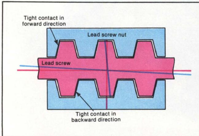
**Fig. 6.** The lead screw nut is off-center relative to the threads of the lead screw to maintain both forward and backward contact. This eliminates mispositioning caused by tolerance problems in these parts. The overlapping centerlines show the center position of the lead screw versus the center position of the nut.
