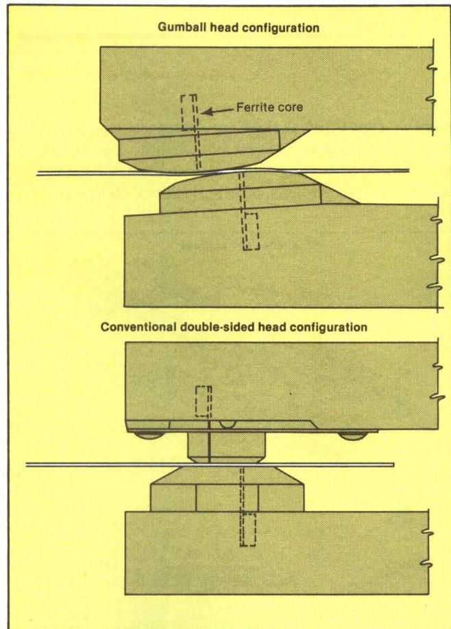
**Fig. 4. The Drivetec gumball heads are spherical to reduce media wear. Unlike conventional heads, there are no sharp edges that can damage the media. The angled positioning of the gumball approach promotes smooth media rotation between the heads while allowing enough proximity to achieve a strong signal.**
