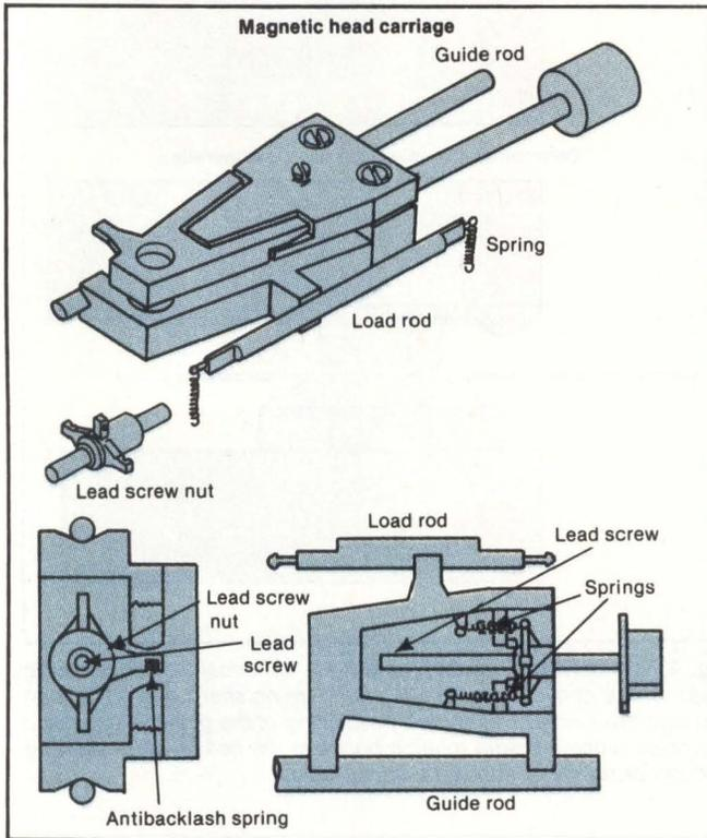
**Fig. 5.** The head carriage assembly (top) has a spring attached to the load rod to align the assembly into the proper orientation for precise head/media alignment. An anti-backlash spring on the lead screw nut decreases the rotational and linear motion of the nut. The underside view of the head carriage assembly shows the placement of the rods, the lead screw, the nut and the two springs that cock the nut.
