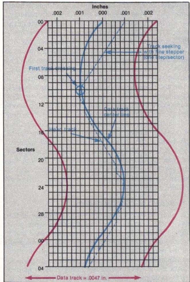
**Fig. 3.** A worst-case condition is indicated by a solid line (the data track) when it is not at a constant radius from the spindle. The dotted line is the track of the head position. If the head is positioned off the data track centerline (top of the grid), it approaches the data centerline at a rate of one step per sector. When it crosses the centerline, the head proceeds to track it to within 0.0001 in., regardless of how the data track centerline fluctuates.
