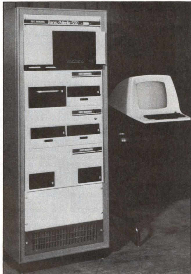
The TM-500 is designed for diskette-to-diskette translation, but can also handle as many as four 800- or 1600-bpi tape drives and as many as two 10M-byte hard disks as I/O media. When the system is used as the front end of vendor-integrated turnkey systems (such as phototypesetters, laser printers and computer-output microfilm), the translated output files are sent directly to the host equipment over one of the asynchronous ports.
