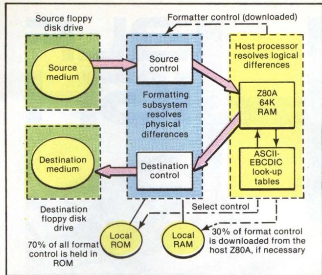
**Fig. 3. The translation process between two floppy disks begins with the formatting subsystem reading the file directory information from the source medium. Formatter control information is down-loaded from the host. Source records are buffered and manipulated in the Z80A under control of BASIC translation programs. Records are then written to the destination medium via the formatting subsystem according to physical requirements.**
