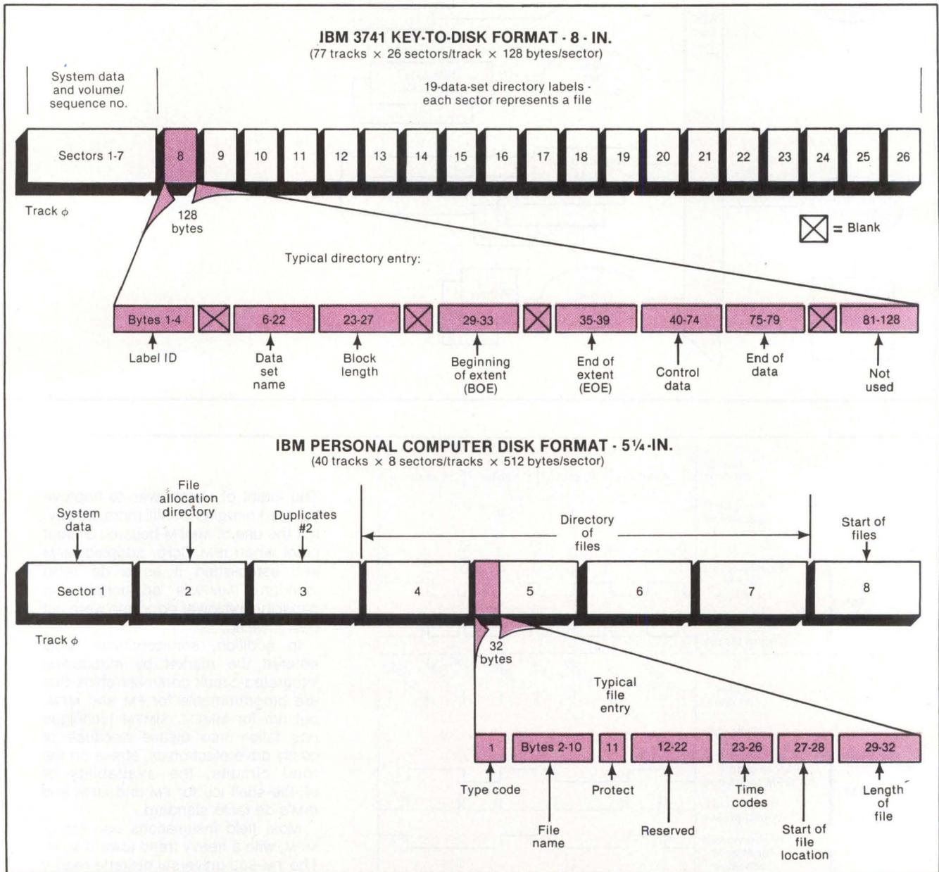
**Formats vary widely, even within IBM.** The above figures illustrate the disk formats of the IBM 3741 (8 in.) and the IBM Personal Computer (5 1/4 in.). The TM-500 resolves the different formats by reading file-directory information from the source, locating occupied files, formatting the destination disk and transferring the source records to the destination disk.
