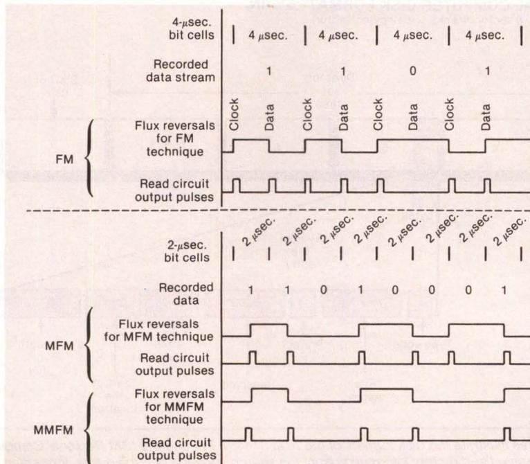
The intent of MMFM was to improve the read margins for still more density, but the use of MMFM became a moot point when IBM Corp. adopted MFM and established it as a de facto standard. MMFM's additional data capacity and lower error rate were not cost-justified.
