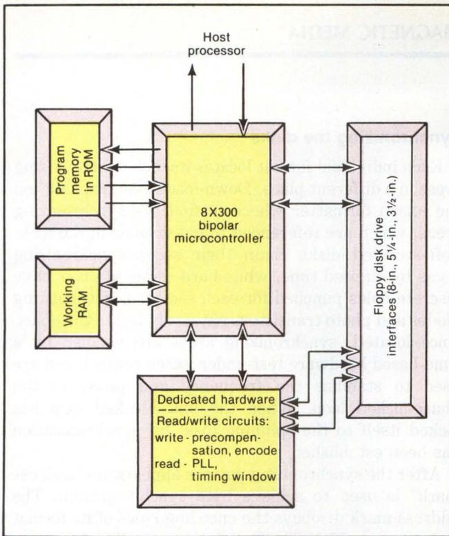
Control files down-loaded to the microcontroller's RAM evoke subroutines stored in ROM. About 70 percent of all formatting control is held in this firmware; the balance is down-loaded from the host's BASIC program when needed and is executed directly from RAM (Fig. 3).
