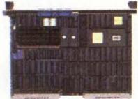
to 4 MB on-card DRAM ▪ One Serial Port ▪ VSB/MVMX32 Memory Expansion Bus.
