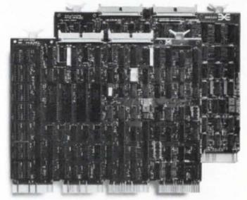
Q-bus embedded dual-density tape controller.
