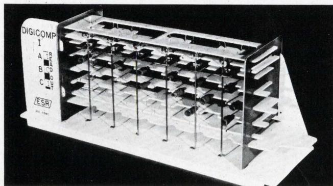
Ingenious mechanical equivalent of an electronic digital computer. Can be "programmed" to perform, individually, every operation of a digital computer. Best thing ever for teaching binary math, how a computer operates, how and why problems must be broken down for machine solution. In kit form—1 hr. to assemble. **\$5.98 Postpaid**
