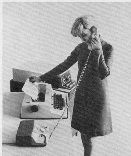
A **Remote Recording** feature, enabling one IBM Magnetic Tape SELECTRIC Typewriter to send information to another, has been announced by the IBM Office Products Division. A telephone data set is utilized in the system for sending exact duplicates of typewritten documents at speeds of up to 150 words per minute.
