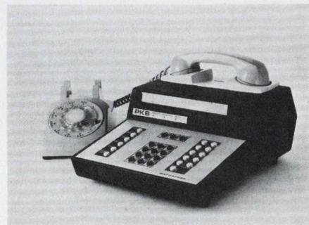
The new system uses an acoustical coupler which sends and receives tone signals through a standard telephone receiver.
