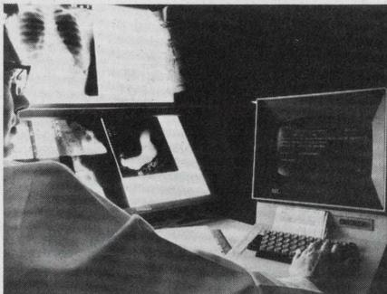
A radiologist prepares an analysis of x-rays on a television-like terminal located in a hospital laboratory. The device is connected to McDonnell Automation Company's computers in Peoria, Ill. The hospital data processing system provides administrative and patient care information.
