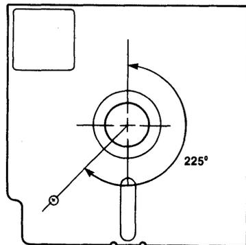
The index hole for the 3M Vydec compatible diskette is located at approximately 225°. Also, notice the extra notch in the lower left corner of the jacket.
