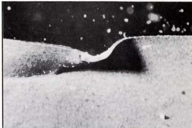
MICROSCOPE VIEW OF A DAMAGED EDGE. AFFECTED AREA EXTENDS ABOUT 15 MILS INTO TAPE.
