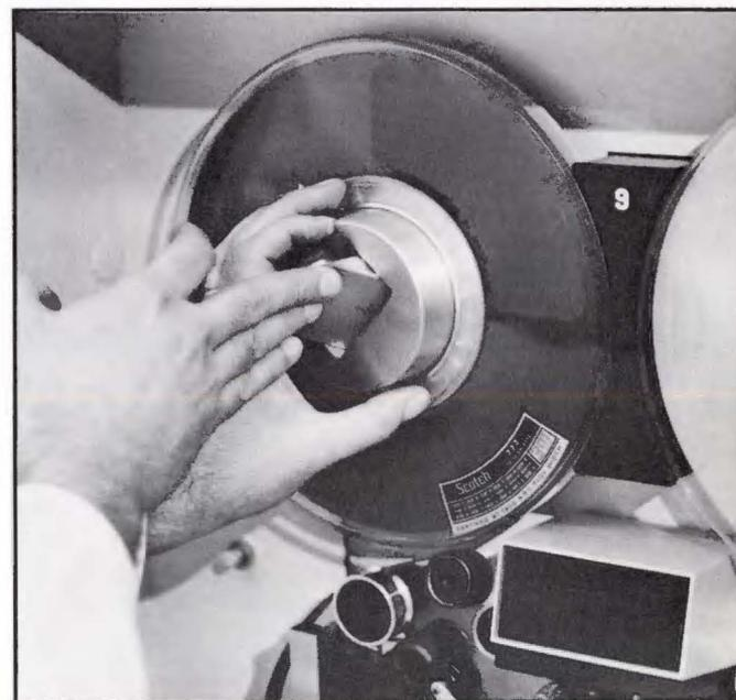
WHEN MOUNTING A REEL ON THE TAPE DRIVE, APPLY PRESSURE TO THE HUB AND NOT THE FLANGES.
