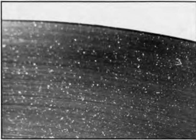
AN ENLARGED VIEW OF DUST CONTAMINATION ON A REEL OF TAPE.
