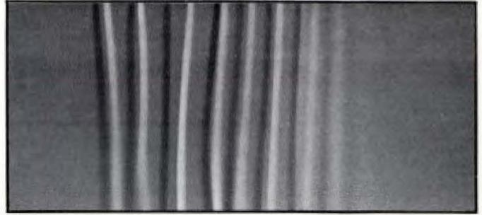
TAPE DAMAGE CAUSED BY CINCHING. THIS 1" LONG STRAND OF ½" COMPUTER TAPE CLEARLY SHOWS THE WASHBOARD-LIKE WRINKLES.
