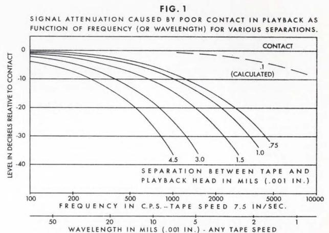
These curves show the attenuation caused by various separations of tape and playback head. On the frequency scale the data are plotted as for a tape speed of 7.5 in./sec., but it should
