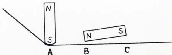
equivalent to an AC erase, but a practical design may involve the use of a small number of poles as an approximation. One head in common use, the type in the Brush "Soundmirror", and the Wilcox Gay "Recordio" uses two magnets arranged to give essentially a three pulse erasure.
