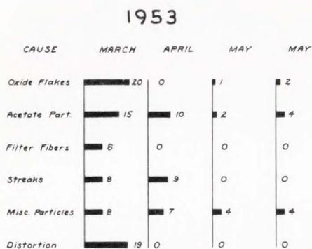
Fig. 3 - This chart shows the number and causes of errors found in four experimental lots of 24 rolls each of tape.
